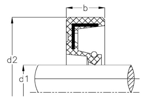
$\begin{array}{ll} b & = 12 \\ d1 & = 85 \\ d2 & = 110 \\ Material = NBR \end{array}$
